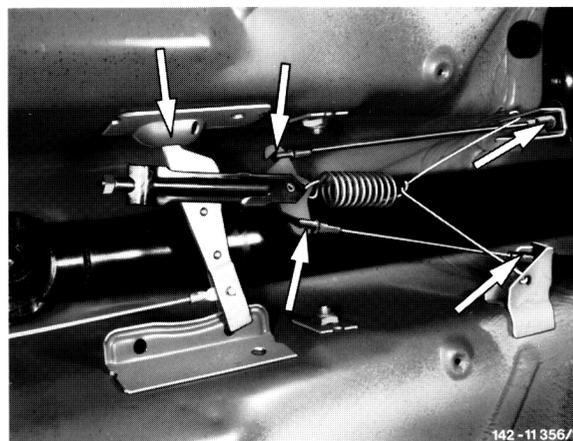
24 Tighten propeller shaft clamping nut on propeller shaft, while paying attention to correct seat of rubber sleeves. Tightening torque on 2-piece propeller shaft 30 - 40 Nm, on 3-piece propeller shaft at front 30 - 40 Nm, at the rear 200 Nm.
