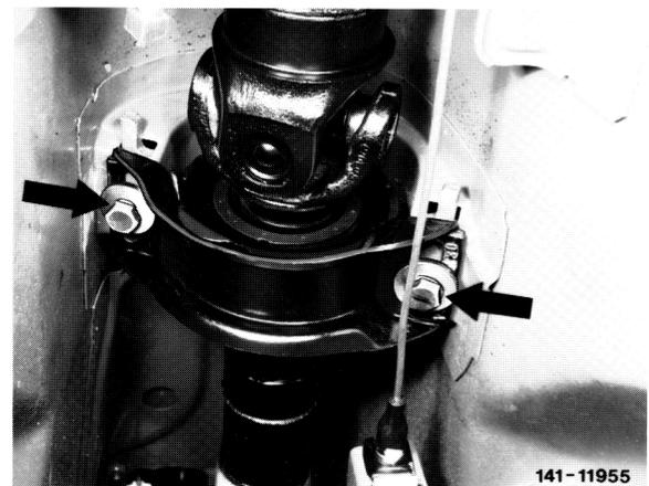
9 Force propeller shaft away from centering pin on transmission and on rear axle. Pull out propeller shaft without vibration damper toward the rear. Make sure that the propeller shaft will not be separated.
