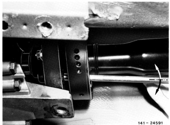
9 Remove propeller shaft from rear axle.
