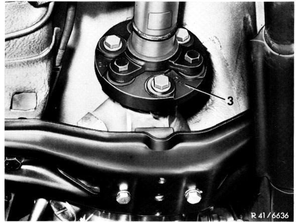
7 Unscrew hex. head screws of propeller shaft intermediate bearing on frame floor.
