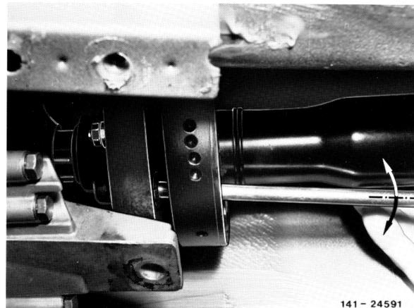
10 Remove propeller shaft from rear axle (arrows).
