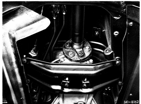
17 Lower transmission and tighten hex. head screws (20) for rear engine mount to 25 Nm.
