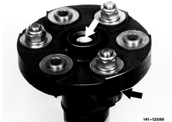
18 Insert front propeller shaft with vibration damper from the front through the bridge and slide onto centering pin on transmission. Push rear and front propeller shaft at clamping connection against each other and slide on centering pin at rear axle.
