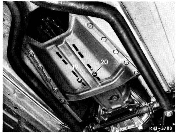
18 Tighten propeller shaft clamping nut to 30 - 40 Nm while paying attention to correct seat of rubber sleeve.
