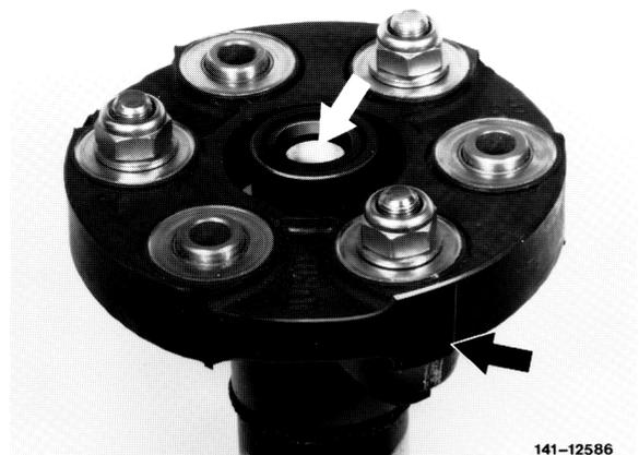
13 Fasten propeller shaft to transmission and to rear axle. Tightening torque of self-locking hex. nuts:
