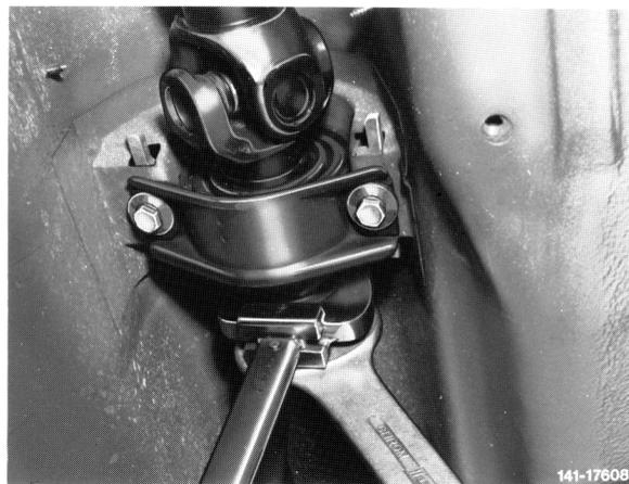
7 Remove front propeller shaft from transmission (arrows).
