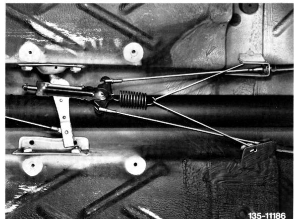
9 Unscrew hex. head screws of propeller shaft intermediate bearing on frame floor.
