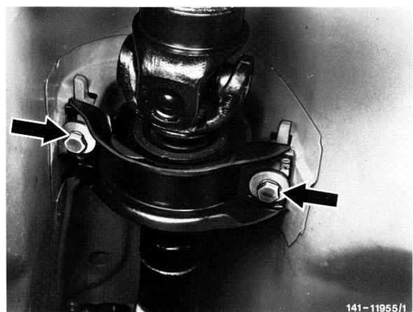
11 Force propeller shaft from centering pin on transmission and rear axle and remove in downward direction. Make sure that propeller shaft will not be separated. On models 126.032/033 starting 09/80 and on models 126.036/037 remove propeller shaft owing to larger flexible couplings of 110 mm dia. angularly through the welded-in cross member.
