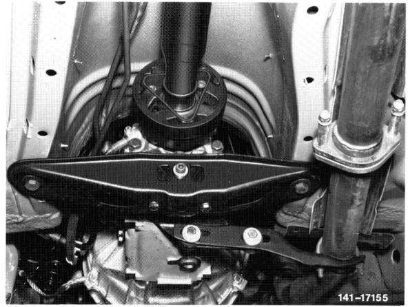
13 Check flexible couplings (12), centering sleeves (10) and propeller shaft intermediate bearing for damage, renew damaged parts.
