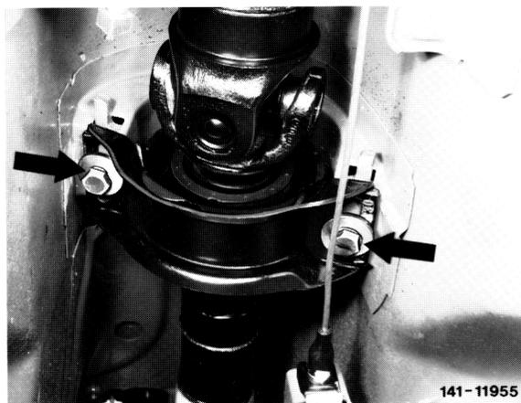
20 Fasten propeller shaft to transmission and rear axle. Tightening torque of self-locking hex. nuts 45 Nm.
