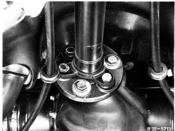
8 Disengage compensating lever of parking brake.
