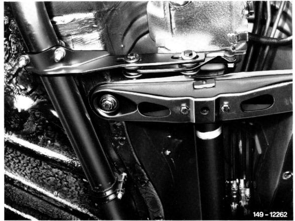
7 Remove propeller shaft on transmission and on rear axle (arrows).
