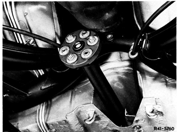
11 On models 107.022/042 starting 09/82 with radially or tangentially soft flexible couplings, loosen the vulcanized centering bushings of flexible coupling prior to pushing back propeller shaft out of flexible coupling (arrows). For this purpose, use a cylindrical mandrel of 10 mm dia. and approx. 150 mm length.
