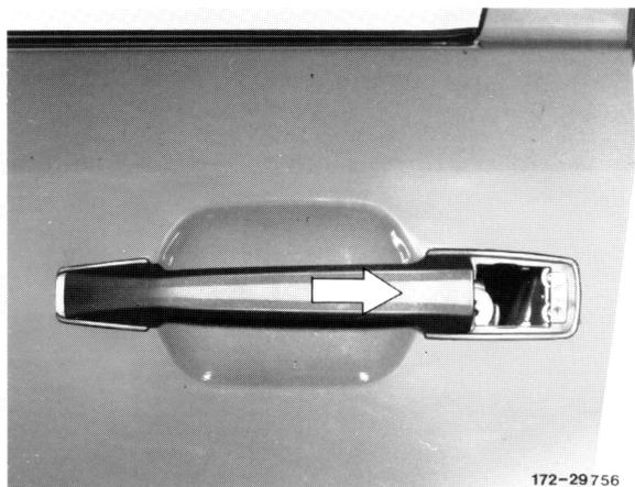
4 Remove grab handle front and rear out of bearing bracket.
