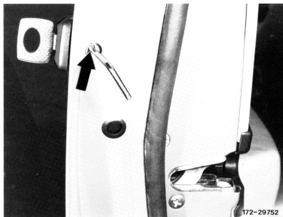
2 Insert door key into locking cylinder, turn approx. 60° to the right while simultaneously forcing locking cylinder toward the rear out of detent on door plate and remove.
