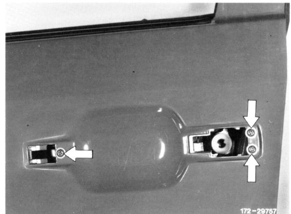
8 Pull bearing bracket forward and remove via assembly opening in door inside plate.
