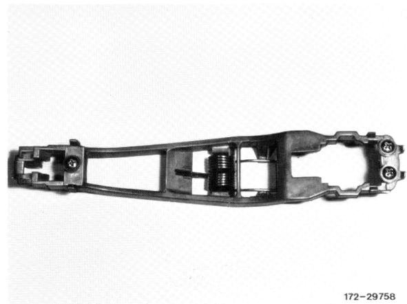
**Note:** When installing grab handle, insert link of rubber rosette between door plate and bearing bracket.
